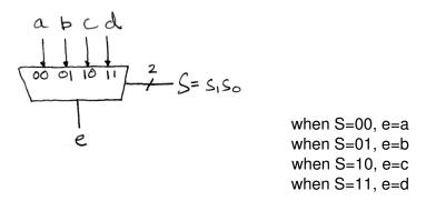
How would we come up with the circuit for this mux? We could start by enumerating the truth-table—in this case the function has 4 single bit data inputs and one 2-bit wide control input, for a total of 6 single bit inputs. The truth-table would have  $2^6$ , or 64 rows. Certainly, a feasible approach. If we where to do this, we would end up with the following logic equation:
