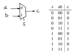
To come up with the logic equation and the associated gate-level circuit diagram we can apply the technique that we studied last lecture. We write the sum-of-products canonical form and simplify through algebraic manipulation. The algebraic steps and final result is shown below. Intuitively this result makes sense; When the control input, s, is a 0, the right hand side of the equation reduces to a, and when it is a 1, the expression reduces to b.
