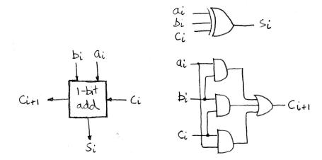
We will not bother creating a special block for the first column of the adder, because anything it can do the 1-bit adder block can do as well. We just need to figure out where to attach the carry-in to the first column. More on this later.
